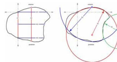
**Figure 4: Engineers compiled data from the CT studies to design the tibia component.**
